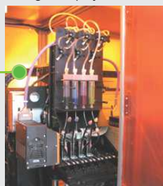
Carriage Part(Inkjet Head/Ink Supply)
