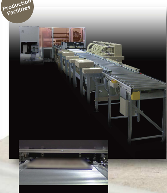
Bring the workpiece flowing on the production line to one side. Positioning with camera
